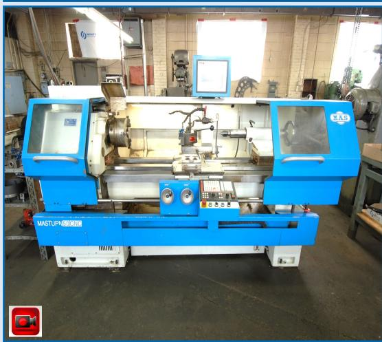
MAS Model MASTURN 50 CNC, Fagor 8055 control, swing over bed 19.7", swing over cross slide 13.8", distance between centers, 59", 10" 3 jaw chuck, travels: X-9.8", Z (carriage slide) – 57", tailstock, 4 station toolpost, follow rest, max workpiece weight 772 lb, 15 HP, sn 278
