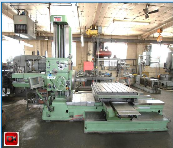
1996 **TOS** Model W100A, 4" spindle, 50 taper, Heidenhain 4 Axis DRO, 49"x49" rotary table, power drawbar, travels: X-63", Y-44", Z-49", W-35", max workpiece weight 6,600 lb, rapid traverse, 110 IPM, 15 HP, sn 4011
